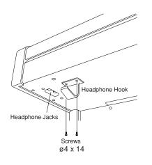
**1.** Attach the Headphone Hook with two screws  $(\emptyset 4 \ge 14)$  to the holes next to the headphone jacks.
